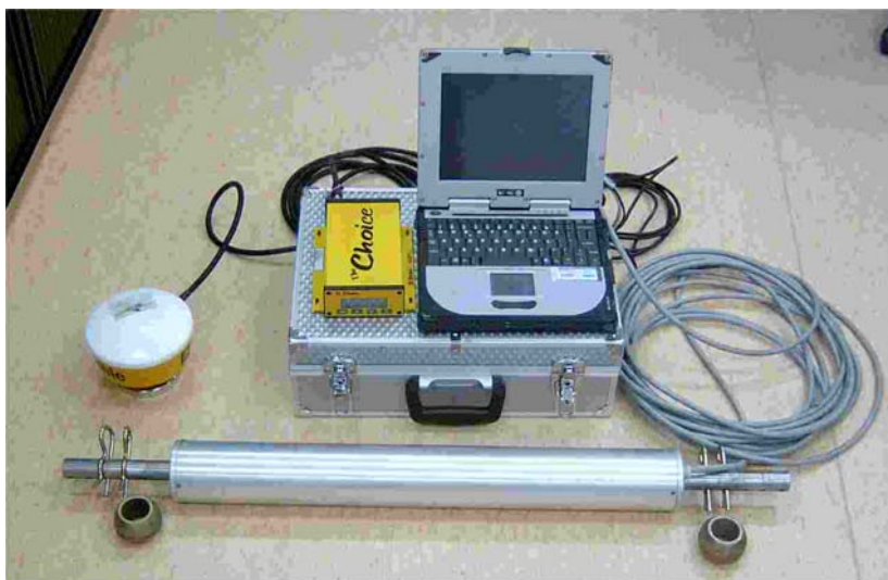
Figure 1. The Mole system of The Soil Company consisting of detector, GPS and laptop.
