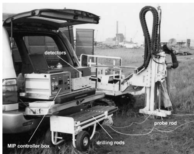
Fig. 1 Field set-up of the MIP system
